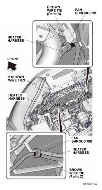
19. Secure the heater harness to the fan shroud ribs with two brown wire ties.
