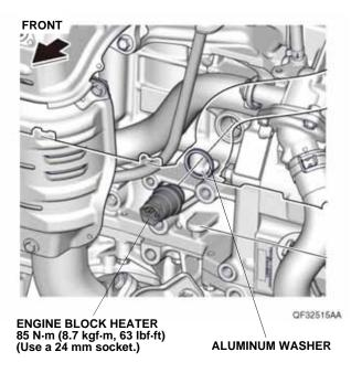
16. Plug the heater harness connector to the engine block heater. Make sure the heater harness connector is fully seated in the engine block heater.
