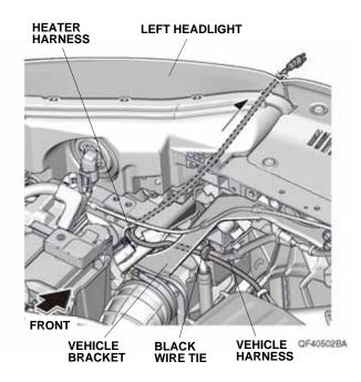
21. Route the heater harness down under the front bumper beam, and secure it to the vehicle harness with one black wire tie at the point D.
