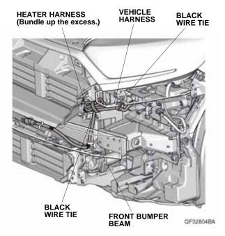
23. Bundle up the excess heater harness, and secure it to the vehicle harness with one black wire tie.
