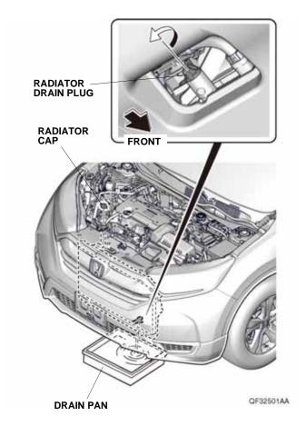
4. Drain the coolant completely, then install the radiator cap.
