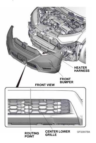
26. Secure the heater harness to the center lower grille with one black wire tie.
