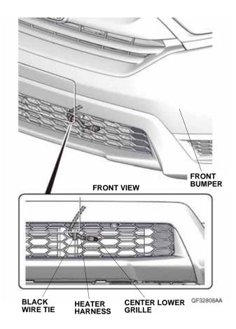
27. Secure the protective cap to the center lower grille as shown, and plug the heater harness connector to the protective cap.
