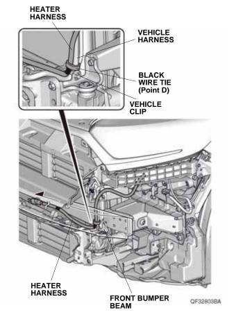
22. Secure the heater harness to the vehicle harness with one black wire tie.
