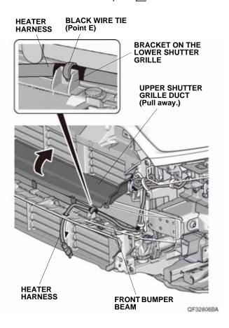
25. With the help of an assistant, bring the front bumper close to the vehicle. Route the heater harness through the center lower grille, then install the front bumper.
