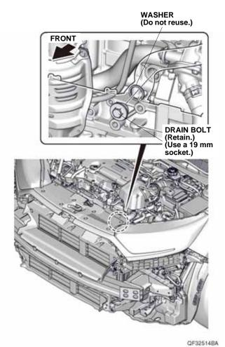
15. Install the engine block heater with the aluminum washer into the bolt hole using a 24 mm socket. Torque the engine block heater to 85 N·m (8.7 kgf·m, 63 lbf·ft).
