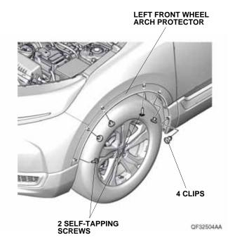
6. Remove the left front wheel arch protector as shown.
