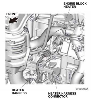
17. Secure the heater harness to the vehicle bracket with one brown wire tie at the point .
