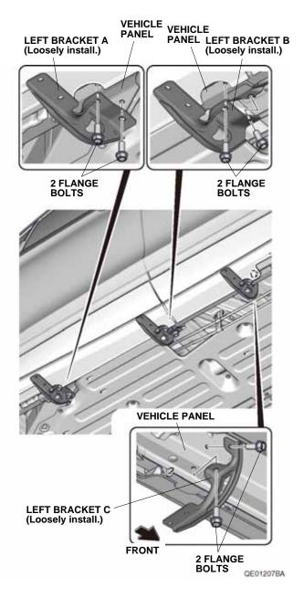
With the help of an assistant, install the left running board to the left bracket A, left bracket B, and left bracket C with six flange bolts. Torque the flange bolts to 27 N·m (20 lb·ft).
