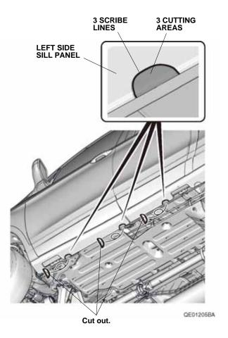
2. Remove the undercoating as shown. Apply touch-up paint where you removed the undercoating and allow it to dry thoroughly.
