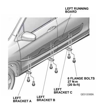
Tighten the six flange bolts loosely installed in step 3. Torque the flange bolts to 27 N·m (20 lb·ft).
