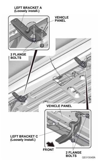
4. With the help of an assistant, install the left running board to the left bracket A and left bracket C with four flange bolts. Torque the flange bolts to 27 N·m (20 lbf·ft).
