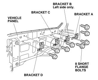
36. Install brackets A, C, and D to the right side of the bed with six short flange bolts. Torque the bolts to 10 N·m (1.0 kgf·m, 7.4 lbf·ft).
