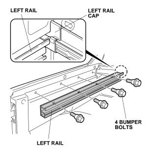
60. Insert two plate nuts into the channel on the left rail.
