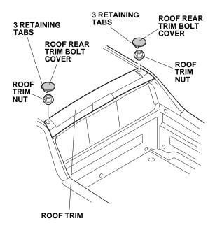
16. Using a plastic trim tool, carefully pry up the front of the roof trim to release three front clips. Start with the left clip, and work your way to the right clip.
