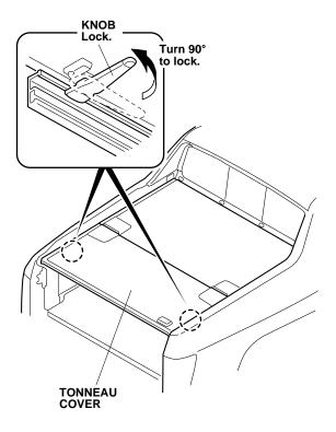
80. Push down on the tonneau cover key cylinder to engage the lock.
