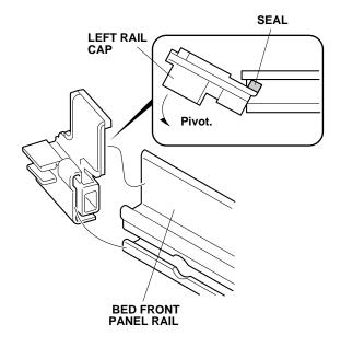
47. Slide the left rail cap onto the bed front panel rail while raising the upper rear towards the front.
