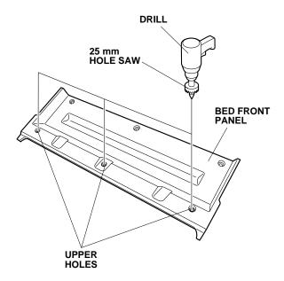
7. While wearing eye protection, drill eight marks on the inside of the bed front panel with a 3 mm drill bit.
