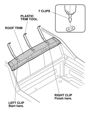
17. Gently lift the front of the roof trim to release four remaining clips.
