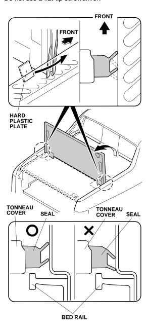
76. Open and close the tailgate several times to position the tonneau cover correctly. Then tighten the four washer-bolts loosely secured in step 73. Torque the washer-bolts to 10 N·m (1.0 kgf·m, 7.4 lbf·ft).
