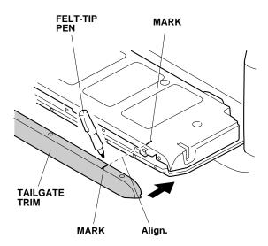
68. Remove the tailgate trim. Measure and cut the tailgate trim as shown.
