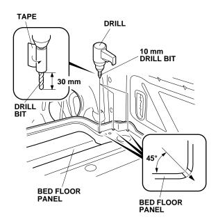
31. Drill three water drainage holes in the same location on the other side of the bed.
