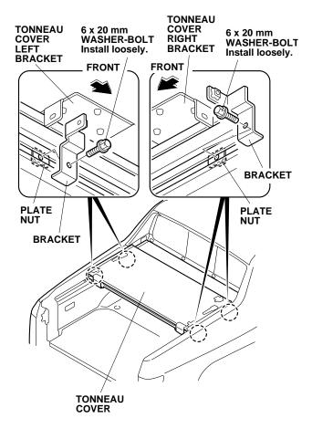
74. Secure the four brackets to the four tonneau cover brackets with 6 x 14 mm washer-bolts. Torque the washer-bolts to 10 N·m (1.0 kgf·m, 7.4 lbf·ft).
