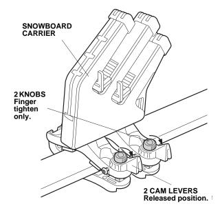
9. Return the cam levers to the original position (turn clockwise).
