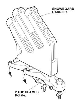
Install two board supports into the snowboard 2. carrier.
