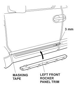
5. While applying light pressure on the trim against the body, carefully remove the adhesive backing strips from the left front rocker panel trim.
