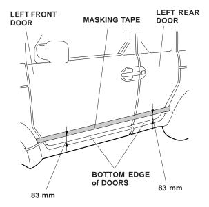
2. Using the alcohol pad, clean the areas where the left front rocker panel trim will attach.
