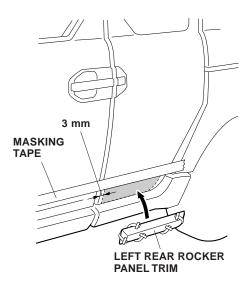
11. While applying light pressure on the trim against the body, carefully remove the adhesive backing from the left rear rocker panel trim.
