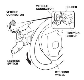
30. Remove two self-tapping screws from the lighting switch. While pushing the retaining tab, slide the lighting switch out of the bracket, and remove it from the steering column. Do not pull on the lever when removing the switch. Do not damage the tab hole in the steering column.
