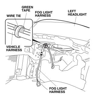
15. Locate and remove the vehicle ground bolt. Secure the fog light harness ground terminal and vehicle ground terminal to the vehicle frame with the vehicle ground bolt just removed.
