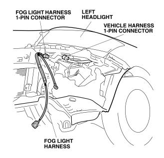
13. Secure one wire tie with clip to the fog light harness at the green tape. Secure the wire tie with clip to the hole in the vehicle frame.
