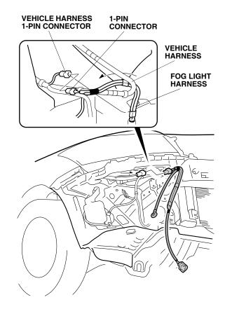
9. Secure one wire tie with clip to the fog light harness at the green tape. Secure the wire tie with clip to the hole in the vehicle frame.
