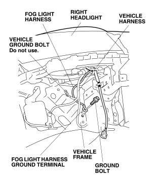
12. On the driver's side of the vehicle, locate the vehicle harness 1-pin connector. Plug the fog light harness 1-pin connector to the vehicle harness 1-pin connector.
