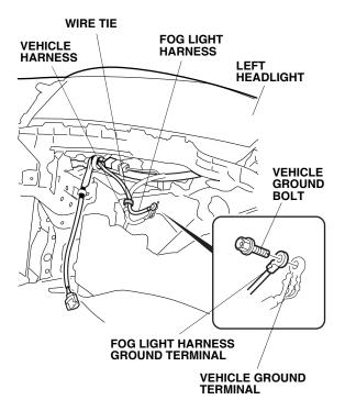
16. Near the ground terminal, secure the fog light harness to the vehicle harness with one wire tie.
