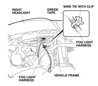
10. Secure the 1-pin connector to the vehicle harness with a wire tie. Secure the fog light harness to the vehicle harness with a wire tie at the green tape.
