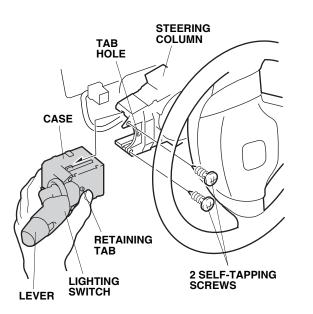
31. Install the new lighting switch into the steering column. Install the two self-tapping screws. Do not push on the lever when installing the case. Push the case into the bracket and set the retaining tab into the tab hole.
