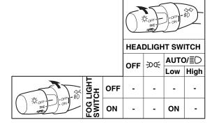
NOTE: The fog light lenses can cloud when the outside temperature is cold; this is normal and should go away in warm weather.
