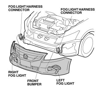
25. Reinstall the front bumper. NOTE: Have an assistant help you when installing the front bumper.
