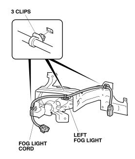
18. Plug the fog light cord 2-pin connector into the left fog light.
