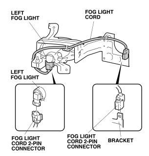
19. Secure the fog light cord 2-pin connector to the bracket.
