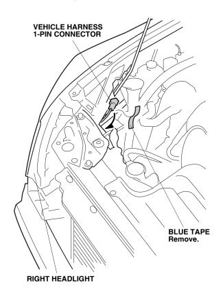
8. Plug the fog light harness 1-pin connector into the vehicle harness 1-pin connector.
