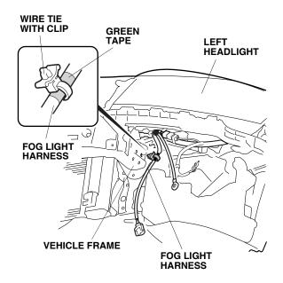
14. Near the 1-pin connector, secure the fog light harness to the vehicle harness with one wire tie at the green tape.
