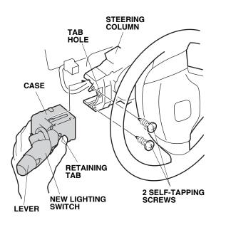
32. Plug the vehicle connector into the new lighting switch.
