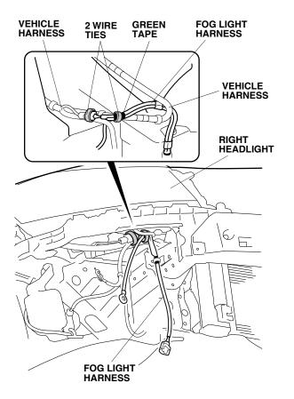
11. Secure the fog light harness ground terminal to the vehicle frame with the supplied ground bolt.
